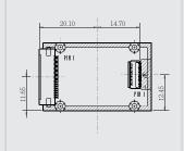
37.00 mm W x 40.90 mm D x 12.00 mm H (Narrow board with one mounting area and connected by molex cable. The engine is separated.)
