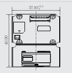
A1 53.00mm W x 40.90mm D x 15.20 mm H (Wide board with three mounting areas and connected by molex cable. The engine is mounted on the board.)
