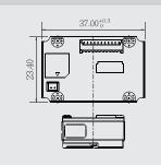
$37.00\ mm$  W x 40.90 mm D x 15.20 mm H (Wide board with one mounting area and connected by molex cable. The engine is mounted on the board.)
