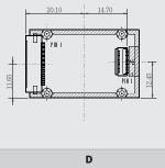
A3 37.00 mm W x 23.40 mm D x 12.00 mm H (Narrow board with one mounting area and connected by molex cable. The engine is separated.)
