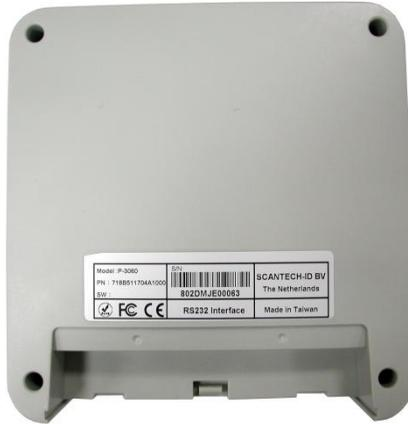
The scanner's serial number is found underneath the bar code label as depicted in the figure above. This official registration number is strictly related to the device. The supplier may ask for this number when the scanner needs servicing.
