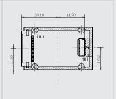
37.00~mm~W~x~23.40~mm~D~x~12.00~mm~H (Narrow board with one mounting area and connected by molex cable. The engine is separated.)
