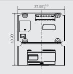
53.00mm W x 40.90mm D x 15.20 mm H (Wide board with three mounting areas and connected by molex cable. The engine is mounted on the board.) 37.00 mm W x 40.90 mm D x 15.20 mm H (Wide board with one mounting area and connected by molex cable. The engine is mounted on the board.)
